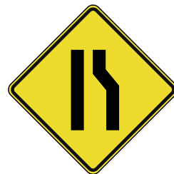
Right lane ends ahead. Prepare to merge.
